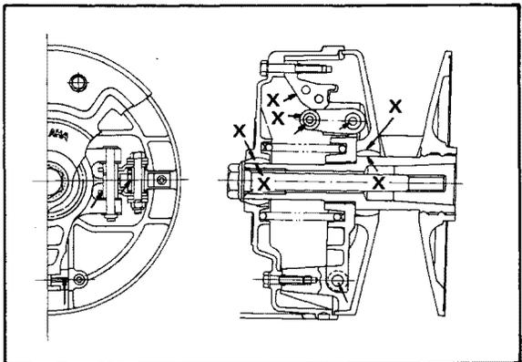
2. Install the bushing and the spider into the sliding sheave. Be sure the bottoms correctly engage the slider.
