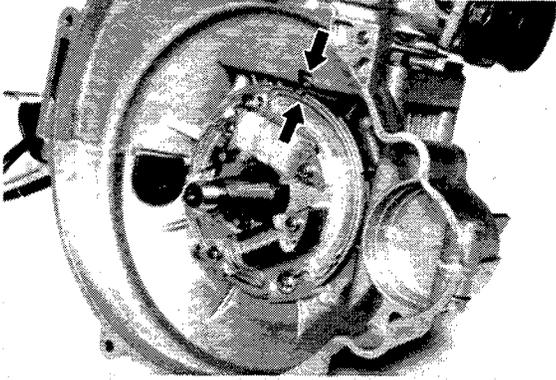
3. Place the woodruff key in the crankshaft, and install the flywheel magneto. The keyway in the magneto must align with the key in the crankshaft. Rap the magneto with a plastic mallet to seat it on the crankshaft.
