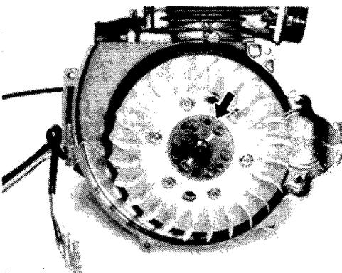
5. Install the flywheel pulley. The two cut-outs on the edge of the pulley must be opposite the holes in the fan. Torque the securing nut to specification.
