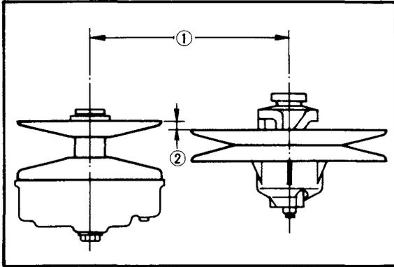
1. Sheave distance:  $266 \pm 2 \text{ mm}$  ( $10.47 \pm 0.08 \text{ in}$ )      2. Sheave offset:  $11 \pm 3 \text{ mm}$  ( $0.43 \pm 0.12 \text{ in}$ )
