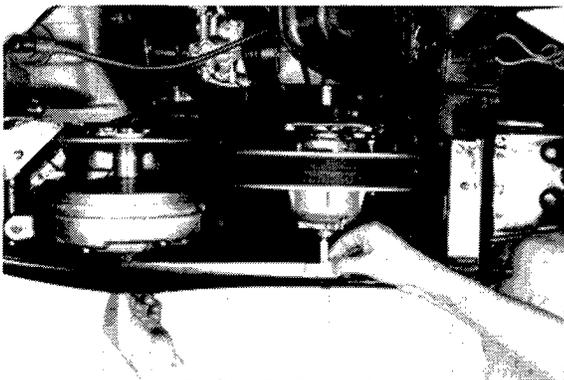
3. If either the center-to-center distance or the offset is not within specification, check the engine mounts. If the engine has been mounted correctly, the engine mounting bracket, the frame, or both are bent. Replace as required.
