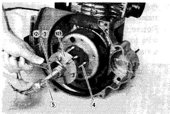
4. Remove the woodruff key from the crankshaft. Remove the two securing screws and remove the coil plate.
