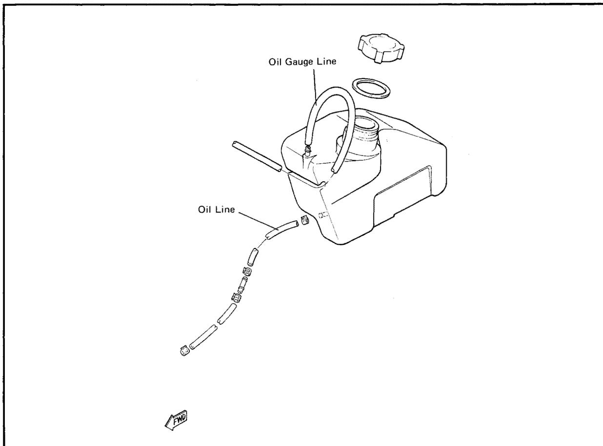
1. Check the oil line from the tank to the pump. It should be free from all obstructions and should not be pinched or
