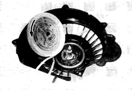
4. Install the drive pawl and the return spring. Hook the spring around the first post on the sheave drum as shown in the photograph.
