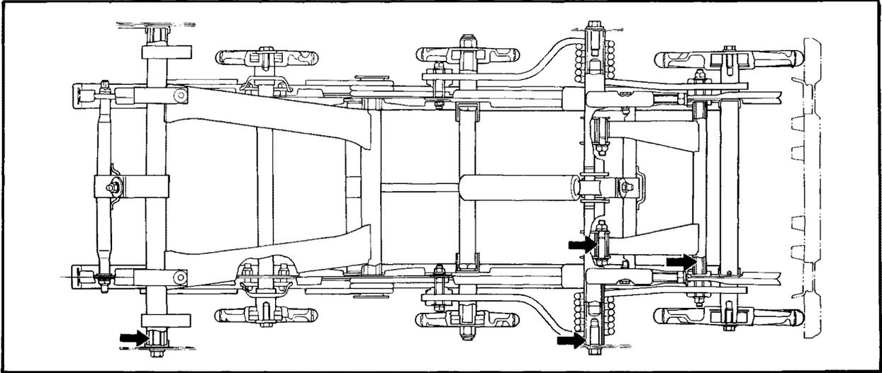
2. Thoroughly grease the axle in the front pivot arm. Tape the end caps in place. This will hold the axle within the pivot arm during installation of the suspension.
