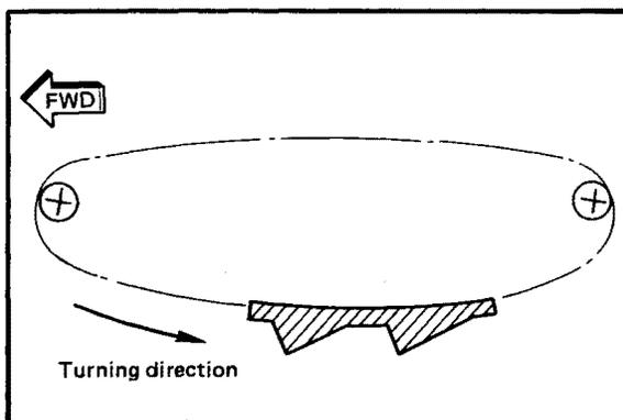
2. Install the axle. Push the threaded end up towards the secondary sheave, then install the splined end into the chain case. Be sure the lugs correctly engage the track.
