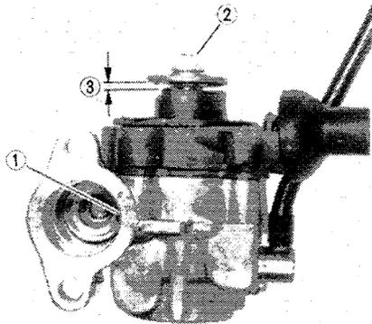
1. Oil pump gear 2. Plunger 3. Minimum pump stroke
