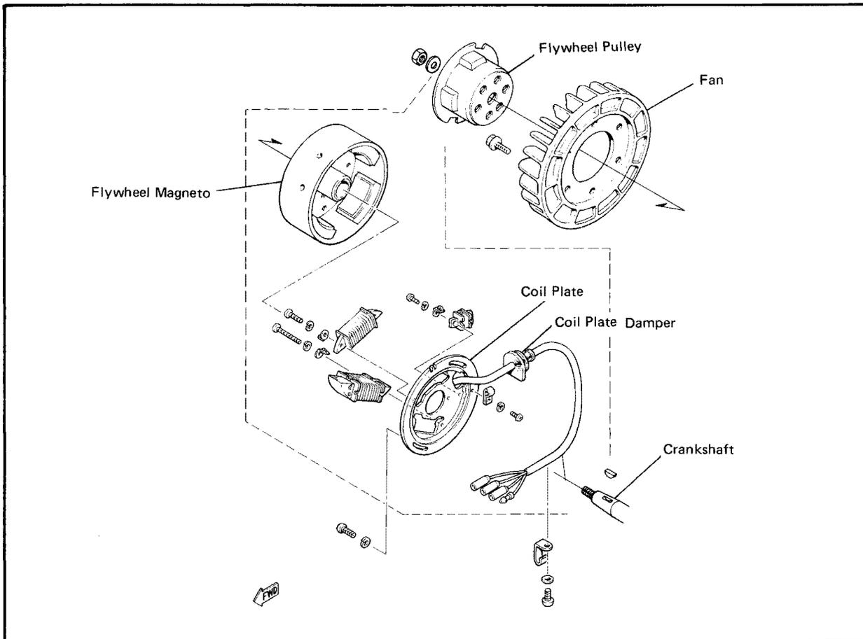
1. Using the rotor holding tool, loosen the securing nut, and remove the flywheel pulley from the magneto.
