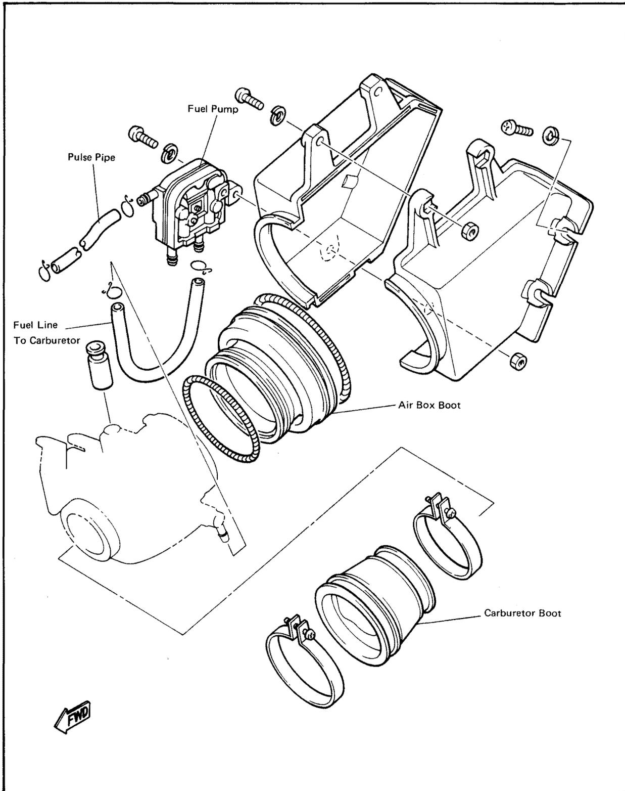
1. Check to see that fuel moves from the fuel tank, to the fuel pump, then to the carburetor. If fuel leaks, replace the components as required.
