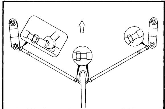
2. The height of the handlebars can be adjusted to suit the rider's preference. After adjusting the handlebars, alternately tighten the four securing bolts. Maintain the specified gap in the steering clamps. Torque the bolts to specification.
