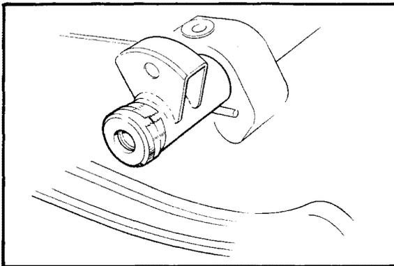
3. Place the suspension in the track, and swing it into place in the chassis. Install both front suspension-mounting bolts. Do not tighten them at this point.
