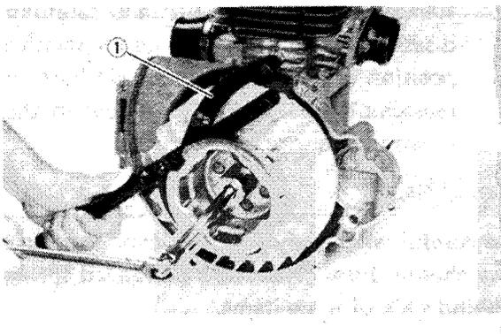
2. Remove the six securing bolts and remove the fan.
