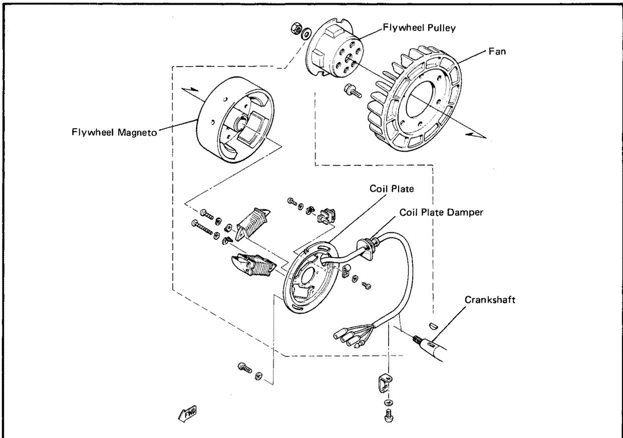
1. Feed the magneto leads through the hole in the crankcase, and secure the damper in the case.
