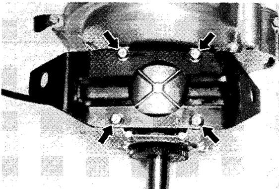
2. Remove the four crankcase bolts. Note the position of the wire bracket. You will have to reinstall it on the same bolt.
