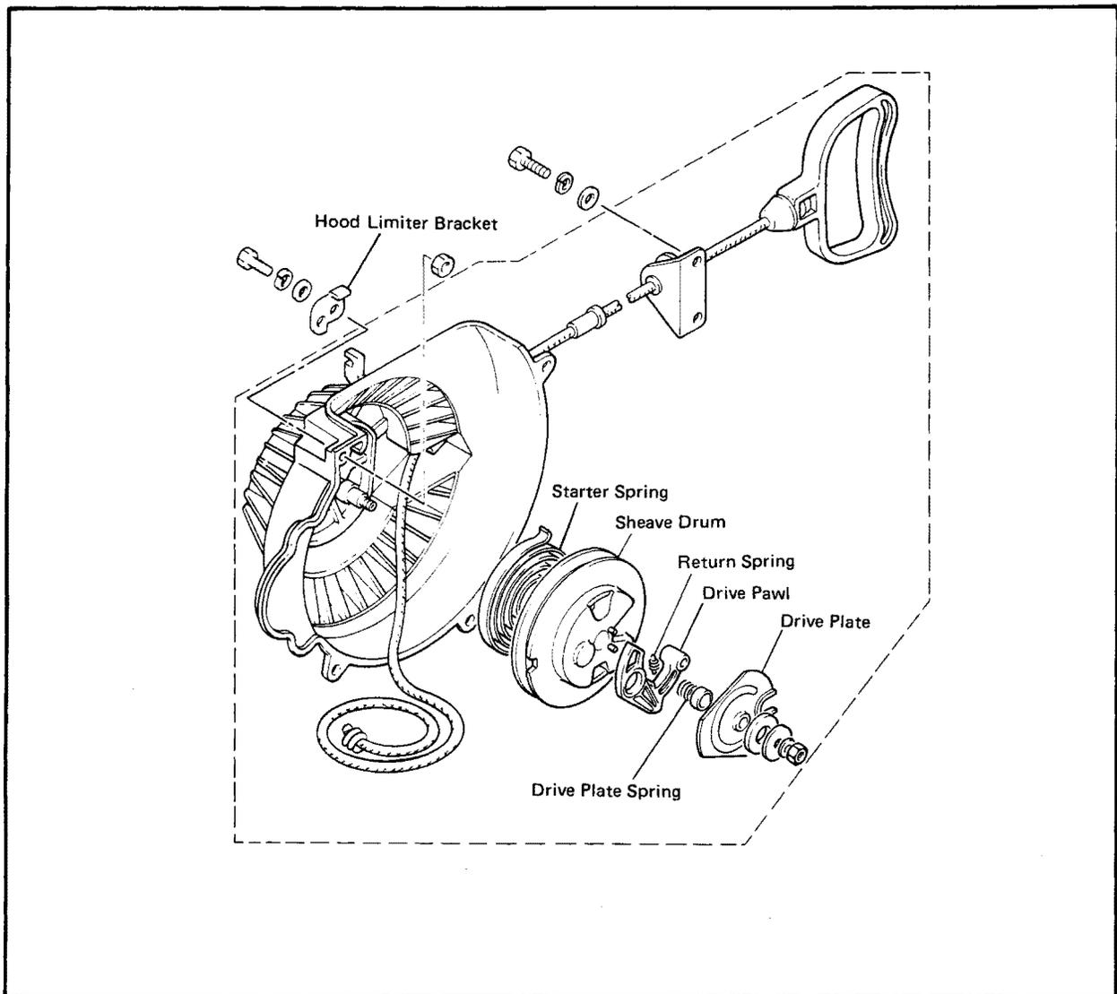
1. Remove the air shroud and the starter from the engine.
