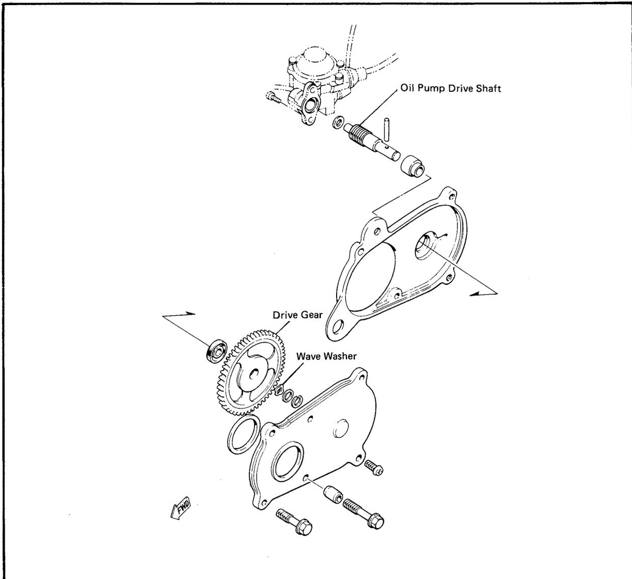
1. Place the washer on the oil pump drive shaft, and insert the drive shaft into the oil pump. Be sure the worm gear correctly engages the oil pump gear in the pump.
