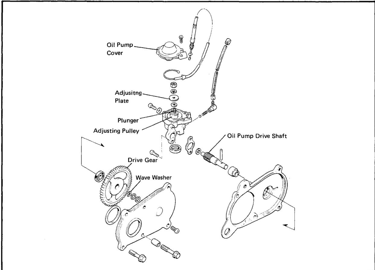
1. Loosen the four gear-case bolts, and remove the gear case/oil pump assembly from the engine.
