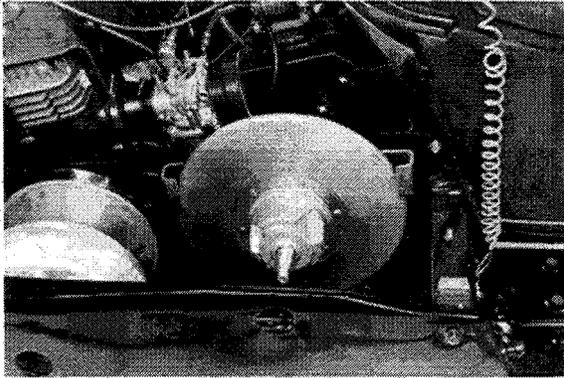
6. Install the key in the jackshaft, and install the fixed sheave. Grease the indicated point.
