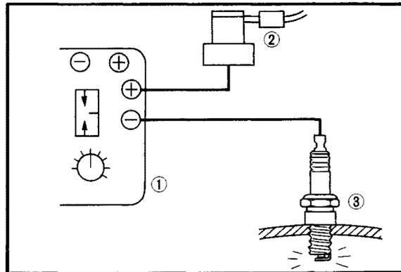
1. Electro-Tester 2. Plug wire from coil 3. Spark plug
