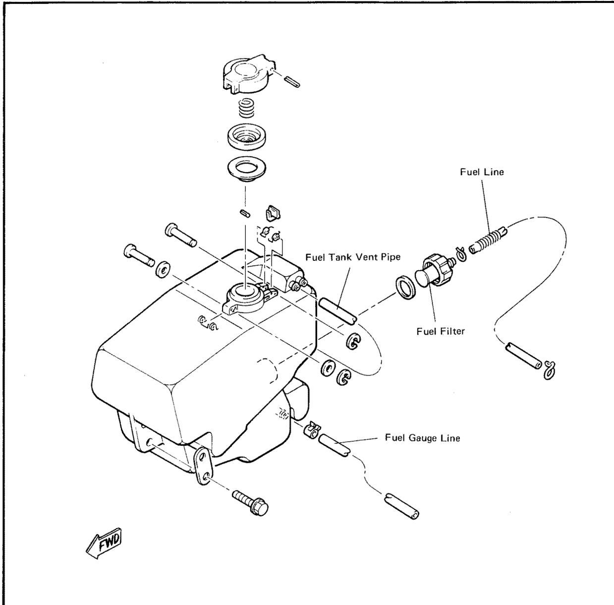
1. Check all lines. If any are cracked, crimped, or damaged in any way, replace them.
