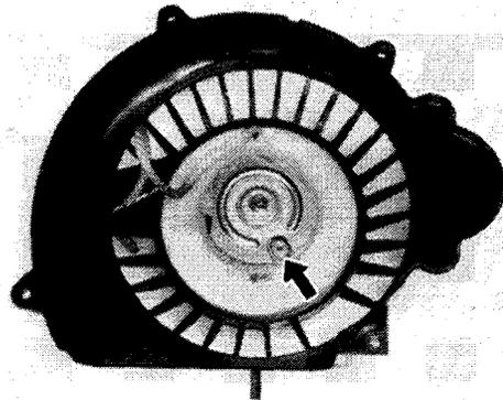
6. Pull about four inches of starter rope from out of the cutout in the sheave drum and form a loop. Rotate the sheave drum five times counterclockwise to preload the starter spring.
