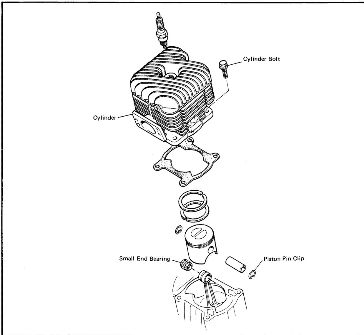
1. Install the piston rings as shown in the illustration.
