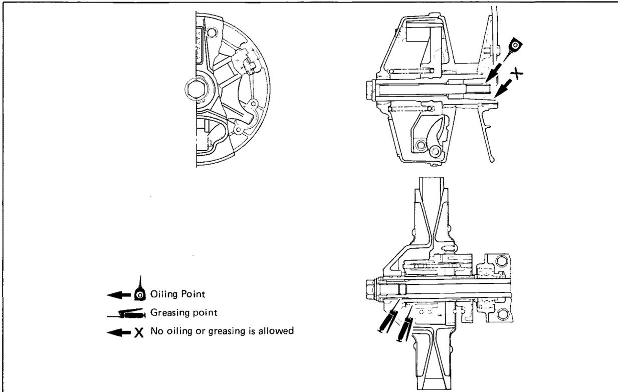
2. Before tightening the fixed sheave, apply thread-locking compound as LOCTITE #640 with PRIMER "T" to the thread portion (bottom four threads) of the spider.
